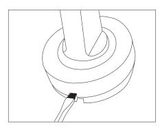
4. Lever the rose cover off the handle. The rose cover will pop off. Carefully slide the loose rose cover off the mini lever.
