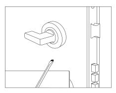
3. To protect the door and hardware from getting damaged, use a small piece of cardboard or something similar and use the screwdriver as a lever.
