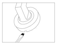
To remove the rose cover, use a flat head screwdriver, ideally the same width as the groove on the bottom of the rose.
