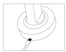
2. Insert the screwdriver into the groove on the side of the rose.
