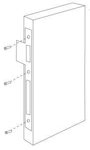
12. Crop out door frame to fit strike plate and dustbox provided using the dustbox as a guide for depth, then insert dustbox behind strike plate and fix to door frame with screws provided.
