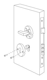
Fit Euro Escutcheon plates around Euro Cylinder and fix to door with screws provided.
