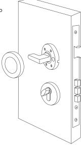
11. Carefully slide the loose rose cover onto the mini lever. Clip on the cover plates to both turns and escutcheons.
